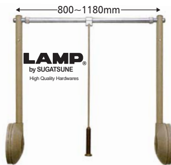
TAW1200 (Double Type) • The double-type model is designed for installation on side walls of a cabinet or closet, using it in full width. • Adjusting the length of the rod is easily done in just one step. Load capacity: Up to 15kg or 33 lbs (evenly distributed)
