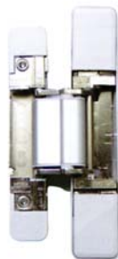
HES3D-V135 3D Adjustable concealed Hinge Door Weight : 40kg (88lbs) 2 pcs Door Thickness : Min.30mm (1-3/16") Max.Door Size : H2000mm x W900mm (H78-47/64" x W35-7/16")
